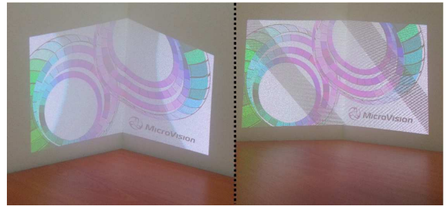
Figure 4. Left: A photograph of the visible key-distortion problem when the separation between the camera and the projector is high. Right: This photograph shows that there is no visible key-distortion effect when the camera is placed close to the pico projector, although the surface is curved.
