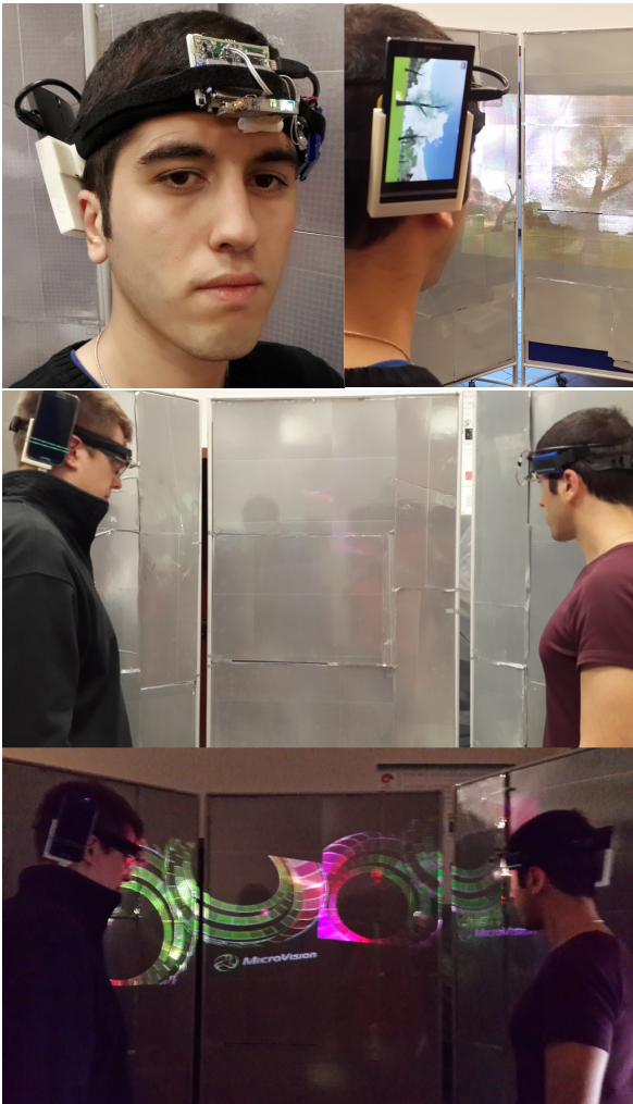
Figure 2. The top picture shows two different photographs of a user with our wearable augmented reality display, the system is composed of a smartphone, an external battery and a pico projector with 3D printed housings. The two photographs(middle and bottom) are showing a scenario where multiple users independently taking benefit of a passive retro-reflective screen without crosstalk.
