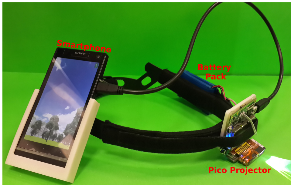
Figure 2.20: A photograph of the hardware device, equipped with a smart phone, a battery and a pico projector. The housing for both items is 3D printed in-house.
