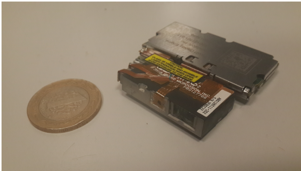
Figure 1.5: A photograph of the photonics module of the laser scanning pico projector from Microvision [1].
