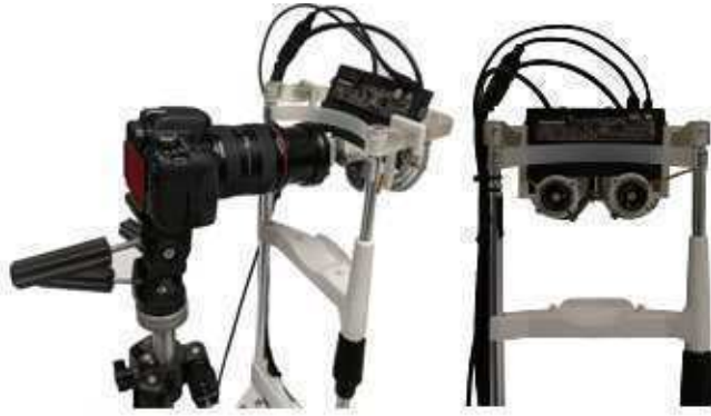
Fig. 6. Prototype hardware and testing configuration Left : Our prototype display with scene capture camera configured to approximate users with normal vision and presbyopia. Right : User side view of our prototype display consisting of vision correcting modules for external world focus adjustments, as well as deformable beamsplitter membranes to drive the focus of the internal display.
