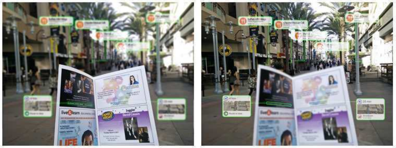
Fig. 2. Mismatch of virtual and real world focus cues in AR for existing conventional AR displays due to all virtual objects placed at a fixed depth plane. [Left] Since the virtual images are placed at a farther depth plane than the book, book appears in focus and the virtual image tags on the book are out of focus [Right] The virtual image tags on the book appear sharp when focused at a farther depth, but now the book is out of focus.
