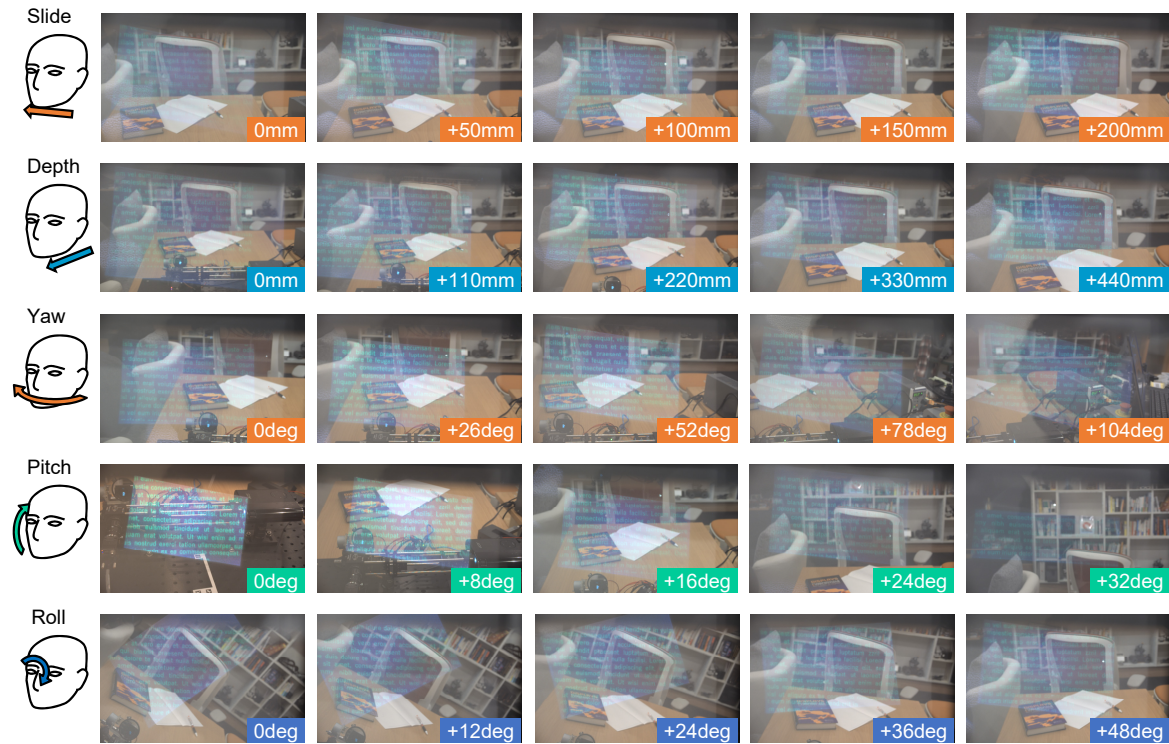
Fig. 14. Qualitative demonstration of the image quality in tracking scenarios with basic head motion sequences. Lengths and angles represent the amount of corresponding motion as offsets. Note that the image projected on the screen keeps the same position except for the visible area due to steered projection.
