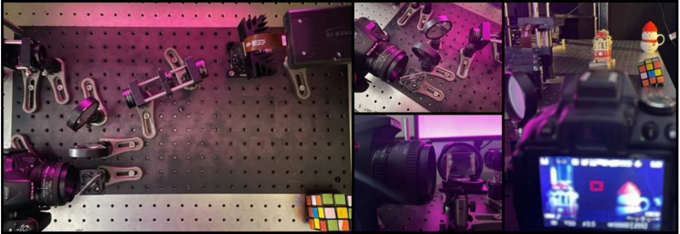
Figure 6: Our proof-of-concept holographic display for Augmented Reality Near-Eye Display application example. Here, we provide various captures of our modified holographic display for AR near-eye display application. We additionally introduce a mirror, eyepiece lens and beam splitter to our display. The camera and the lens imitate the user's view with changing focus cues. The right image demonstrates the actual scene that we used in our captures. The Rubik's Cube, train, and snowman are located 45 cm, 65 cm, and 100 cm away from the camera.
