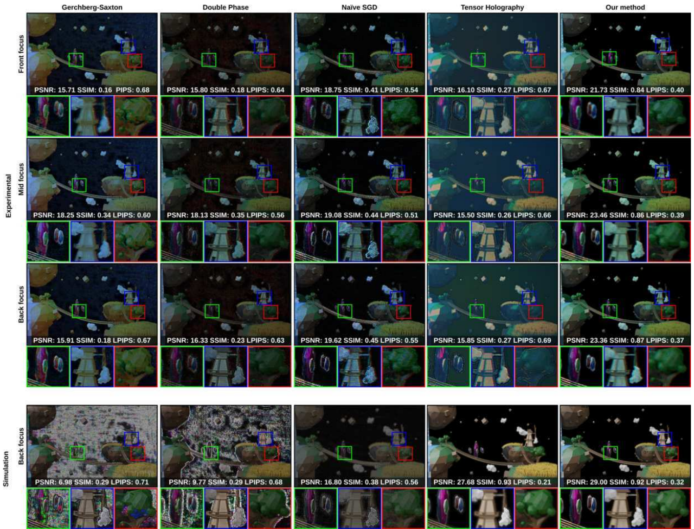
Figure 5: Comparison of methods. We show actual captures from our holographic display for three different focuses in the top three rows. In addition, a result from a simulation focusing on the back is presented in the bottom row. All the captures from our holographic display use 20 ms exposure time. We tune laser powers for each case highlighted per column to get to the best possible image quality in the corresponding case. These cases include the following items from left to right: (1) optimizing multiplane holograms using the Gerchberg-Saxton method [41] with our targeting scheme, (2) optimizing multiplane holograms using the Double Phase method [13] with our targeting scheme, (3) optimizing multiplane holograms using Stochastic-Gradient Descent (SGD) [38] with naïve targeting where defocus parts are painted with black pixels in the target images. This specific case approximates the naïve version of the work by Peng et al. [28], Chakravarthula et al. [6] and Choi et al. [9] closely, (4) Optimizing a continuous depth hologram using the state-of-the-art method, tensor holography [31], and (5) optimizing a multiplane hologram using our method uses SGD and use an update rule inspired from Double Phase method. In actual captured results and simulations, our method distinguishes itself as the contrast preserving, fringe artifacts free and high-visual quality method.
