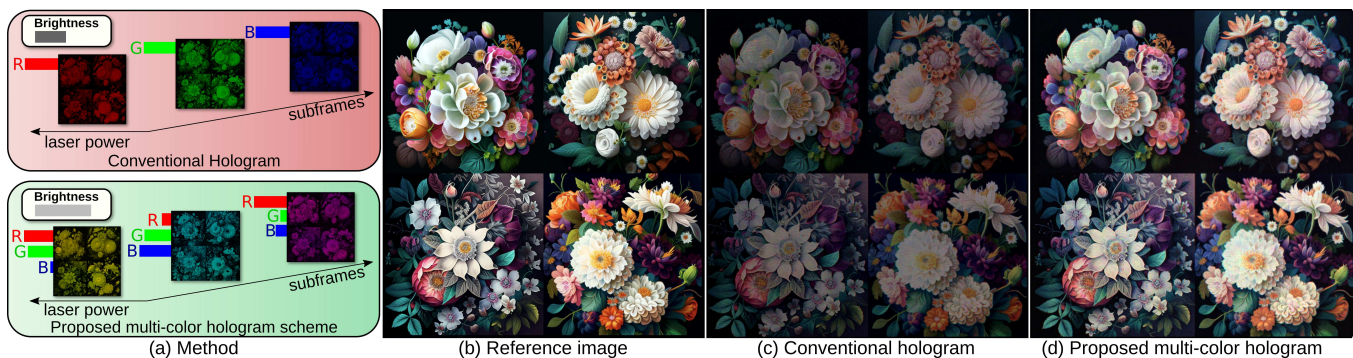
Figure 1: Our framework simultaneously uses multiple laser light sources to support brighter images in holographic displays. (a) Conventional holograms display full-color images using single-color holograms, each dedicated to a color channel and illuminated by a single laser light source. Our method instead optimizes multi-color holograms, each lit by and modulates multiple laser light sources. Given a reference image (b), photographs captured from a holographic display prototype with an 80 ms exposure: (c) A conventional hologram reconstructs an image with limited brightness, and (d) A multi-color hologram reconstructs a brighter image (Source image: Midjourney, Link: Github:complight/image).
