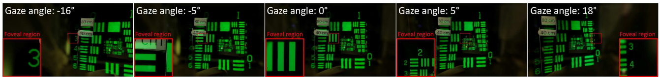
Fig. 15. Display results of different gaze angles with the optical bench prototype. Note that the virtual scene was located at the center view and independent of the gaze angle, and that the foveal region is always located at the center.
