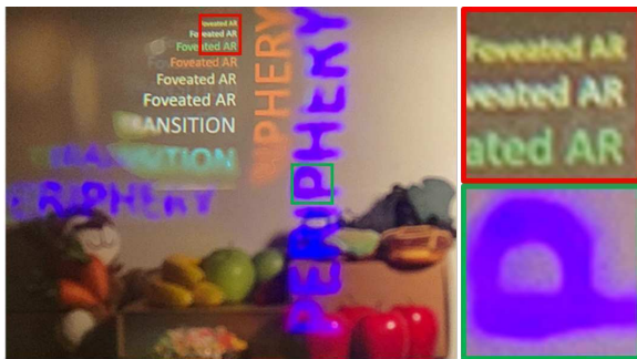
Fig. 17. Display photographed through the display of the wearable prototype. The top, red inset shows a detail from the foveal region and the lower, green inset is from the peripheral region. Note that the smaller projector used in the wearable prototype has narrower light cone angle and worse color representation which led to smaller FOV ( 77^\circ \times 53^\circ ) and severe color mismatch.
