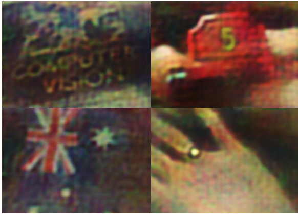
Fig. 5. Reconstructions from our lensless camera prototype trained using our RGB model. Our optical element consists of a thick holographic diffuser (0.76mm) with bulk scattering, leading to a degradation in image quality.
