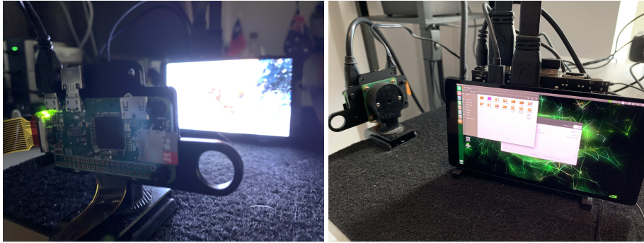
Fig. 3. Photos of our lensless camera prototype. The camera is aimed at the display to capture paired training examples. The paired training examples are used to train our learned image reconstruction model.
